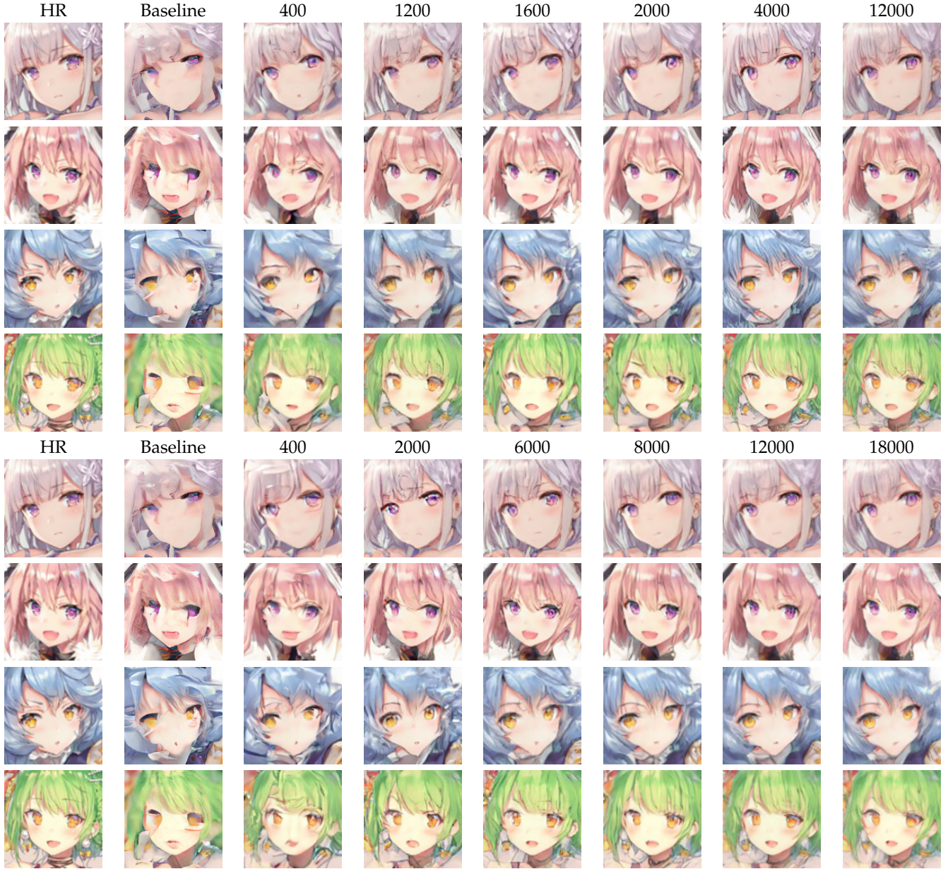
Fig. 3: The leftmost column shows the HR images and the second column shows SR image using the pretrained model without fine-tuning. Other columns show SR images with different fine-tuning steps. SR images above are fine-tuned with L1 loss, and below are fine-tuned with L2 loss.
