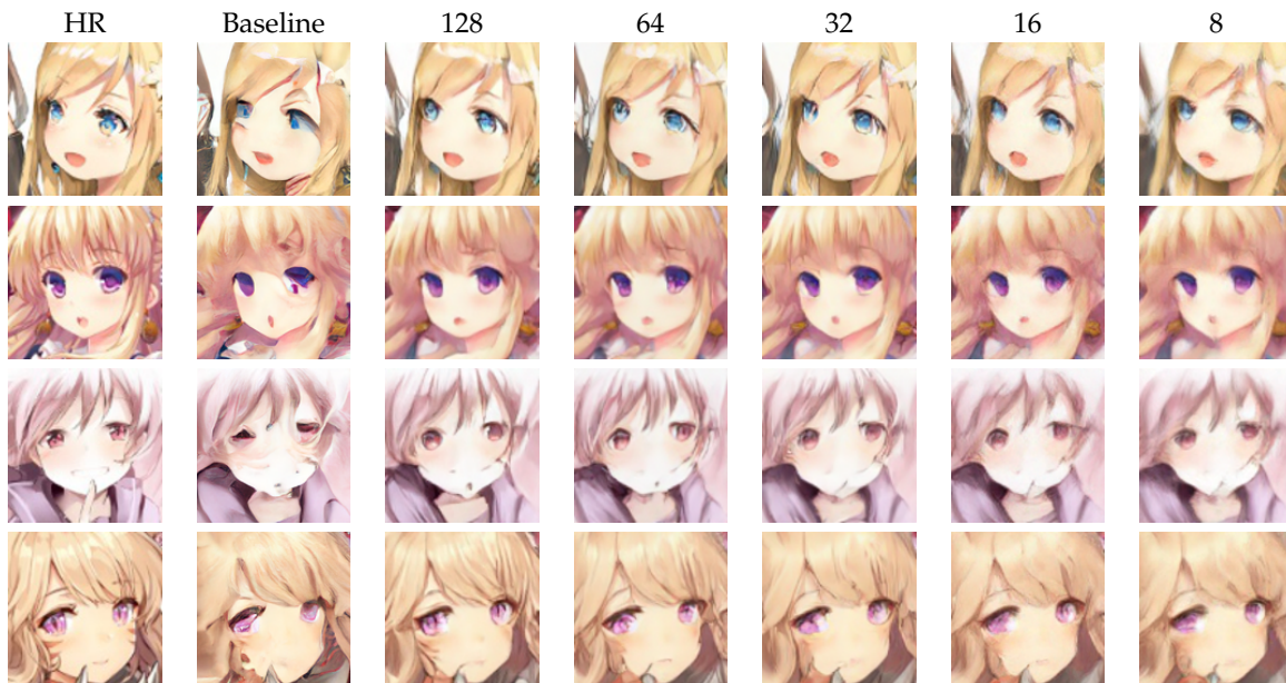
Fig. 4: The leftmost column shows the HR images and the second column shows SR image using the pretrained model without fine-tuning. Other columns show SR results fine-tuned on different amount of data. All SR images are fine-tuned 2000 steps with L1 loss.
